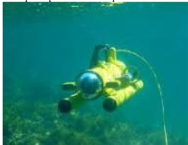
Payloads for underwater SAR use include cameras and sonars. Video cameras are mounted on ROVs or can be attached to poles that can be dipped along piers or from boats to look for victims.
