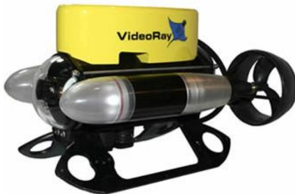
The ROV is also known as an Unmanned Underwater Vehicle or UUV. An ROV is tethered, meaning that it is attached to a
